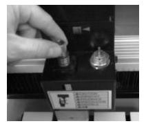
5. Ensure that the nosecone is turned "counter-clockwise" almost all the way down. The ratchet sound heard from the ball clicking into the indentations on the micrometer ring will disappear if you turn the ring to far.
