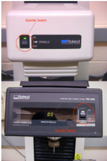
Spindle Switches: PNC 2500 top, PNC 3100 bottom
