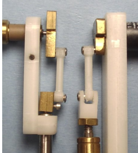
Figure 38. Left: Original Design. Right: Yoke Design
