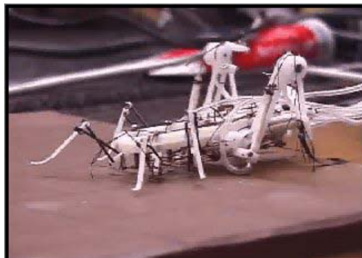
Figure 76. Robot with All Actuators Relaxed
