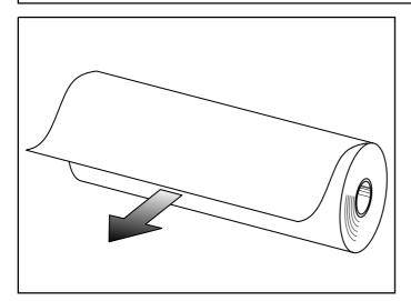
Pull out the amount to be used for printing. This can be performed most easily if you set the sheet on the PC-60 after powering off.
