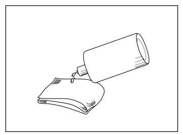
Wipe the surface of the sheet strongly with a cloth soaked in alcohol to remove the dust and oil.
