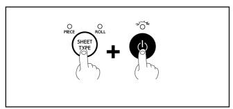
While pressing the SHEET TY PE key, turn on the sub power by pressing key.
