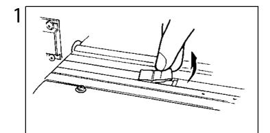
Remove the old cleaning pad from its right side.
