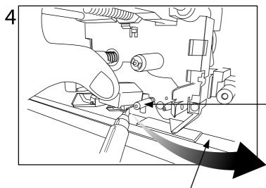
Clean the edge of the printing head with the cleaning pen. It is not necessary to clean the bottom part.
