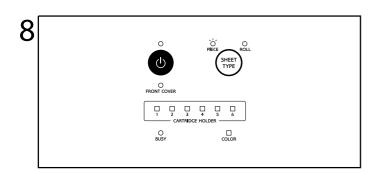
When the front cover is closed, head cleaning begins. Head cleaning is finished when the BUSY LED goes dark and the PIECE LED flashes.
