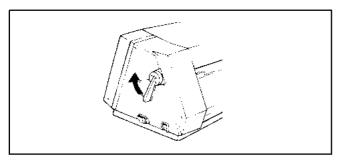
Raise the sheet loading lever. Unload the sheet from the machine.
