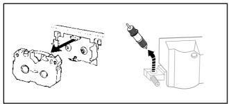
Take out the ink ribbon cartridge and remove the blade holder.
