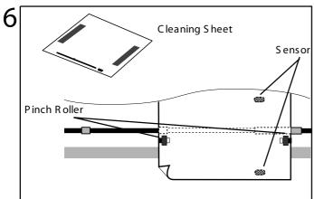
Position the material, the pinch rollers, and the grit rollers at the locations shown above.
