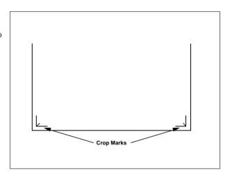
Move the **CARRIAGE** with cursor keys so that the pen tip will come right onto the corner of the right lower crop mark when pushing it down with your finger.
