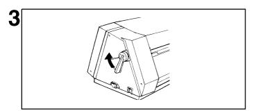
Raise the sheet loading lever. Unload the sheet from the machine.
