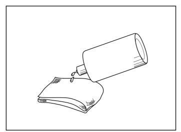
Wipe the surface of the sheet strongly with the cloth soaked up with alcohol to remove dust and oil.
