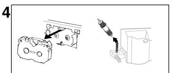
Take out the ink ribbon cartridge and remove the blade holder.
