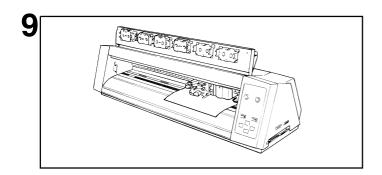
When cleaning is finished, raise the sheet loading lever and remove the sheet.
