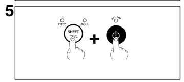
While pressing the SHEET TYPE key, turn on the sub power by pressing key.
