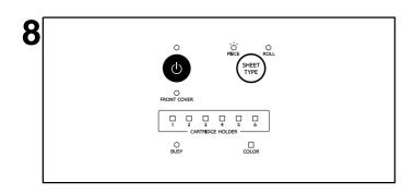
When the front cover is closed, head cleaning starts. Head cleaning is finished when the BUSY LED goes dark and the PIECE LED flashes.
