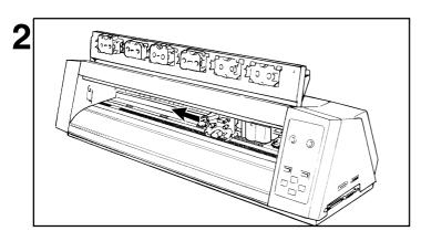
Open the front cover and move the printing head to the left side of the machine.
