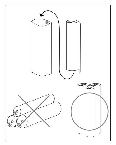
Keep the roll sheet inside the vinyl bag when it is not being used. Try to avoid dust from sticking to the surface of the sheet as much as possible.
