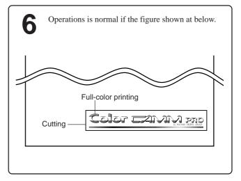
After the operation check has finished, raising the sheet loading lever cancels the operation check mode. After that, the unit operates as it does when the power has been switched on in the normal manner.
