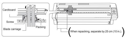
When repacking, tighten the screw in place while lifting it up so as to sandwich the cardboard as shown in the figure. Make sure the blade carriage does not move up or down.
