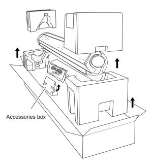
**CAUTION** Unpacking, installing, or relocating the unit are operations which must be carried out by two or more persons holding the unit at its bottom surface on the left and right sides. Failure to do so may result in dropping the unit, leading to injury.
