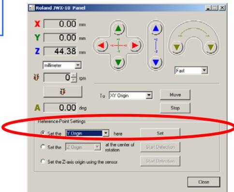
Set the Y-Origin at this location using the setting shown. After pressing the “Set” button, the Y-Origin will now read 0.00 mm.
