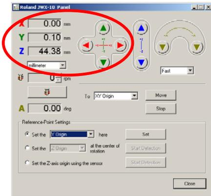
Move the tool half of the measured offset in the Y-direction only.
