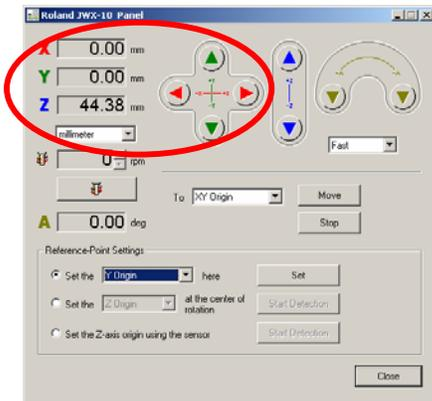
Move the tool to the X & Y Origin Position.
