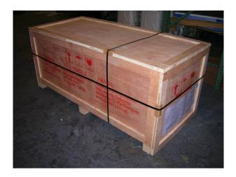
2: Locate the two metal banding strips on the outside of the crate and remove by cutting with a pair of metal snips. Please use caution when cutting because these straps may have pressure and will snap when cut.
