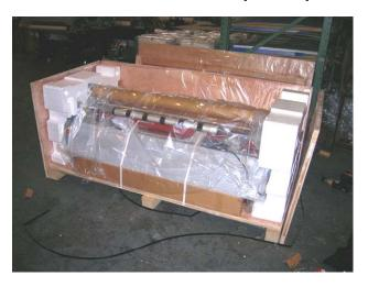
5: Cut the center two white plastic strapping that hold the laminator to the bottom of the packing crate.
