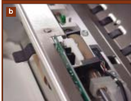
Figure 1a and b: Flag hold-downs were made in lots of 100 on a Stratasys FDM system. Figure 1b shows the flag hold-down in use.
