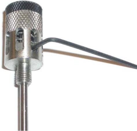
Install diamond scribe tool into spring loaded adaptor using included wrench.
