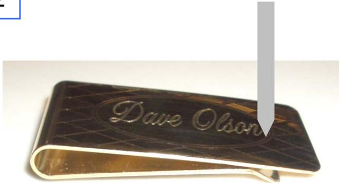
When using irregular shaped objects, you must set the correct tool height at the lowest point.
