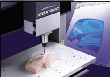
Precision X,Y,Z motion control enables you to create smooth detailed prototypes from a wide array of non-proprietary materials.
