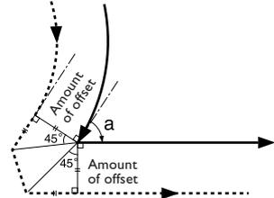
From an arc to an arc
