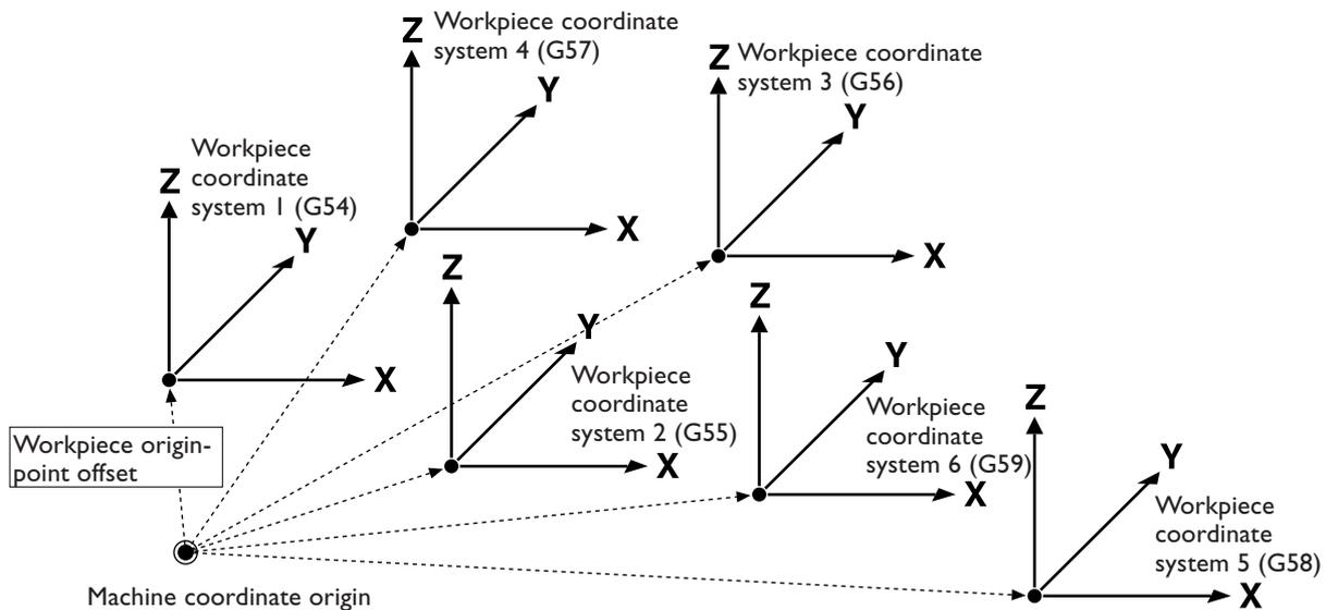
Note, however, that the state shown in the figure above is obtained when EXOFS is zero. EXOFS (the external workpiece origin-point offset) shifts the six workpiece coordinate systems as a group. The setting for EXOFS is made on the modeling machine. (It can also be specified using G10.)
