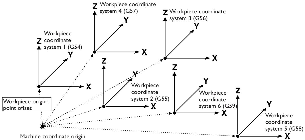
The locations of the six workpiece coordinate systems (that is, the six workpiece origin-point offsets) are set on the modeling machine.
