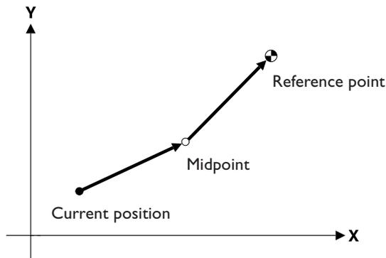
The midpoint is determined as follows. When X *x*, Y *y*, Z *z* is omitted, the coordinate of a G28 code executed in a previous block is used. Also, when no coordinate at all has been specified for a particular axis, no movement along that axis is performed. An example is shown below.
