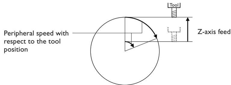
When the Z axis is at its highest position, the rotary axis unit rotates at maximum speed irrespective of any specified F code.
