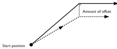
The following explanation describes the tool path when tool-diameter offset is started.
