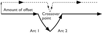
In this case, a crossover point exists on the tool path for arcs 1 and 2.
