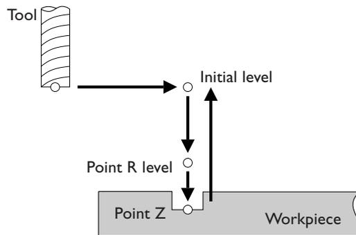
Cutting is performed at the spindle speed and feed rate that have been specified.
