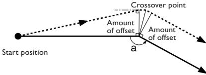
**From a line to an arc (Type B)**
