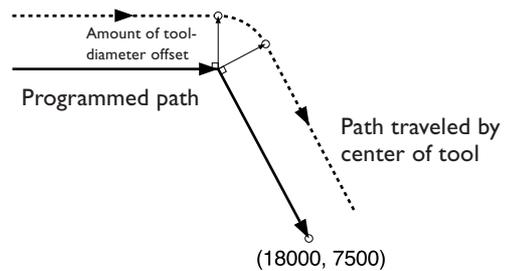
G39 is a word that is effective only within the block where it is specified. G39 functions only once, and circular interpolation is canceled in the next and subsequent blocks. G39 does not affect G00, G01, G02, or G03.
