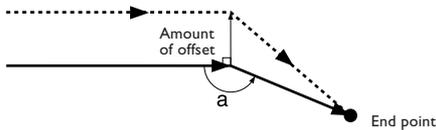
From an arc to a line (Type A)
