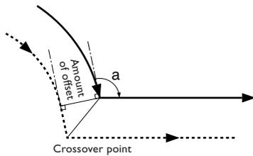
From an arc to an arc
