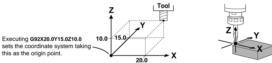
Move the tool to the starting point assumed by the program before sending the data. This example assumes that the front-left corner of the workpiece is to be specified as the origin point for the workpiece coordinate system.
