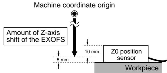
The thickness of the Z0 sensor may vary slightly due to conditions of temperature and humidity. The sensor thickness can also be used to make fine adjustments when high accuracy is required. Because cutting depth is affected, an incorrect setting may result in breakage of the tool.
