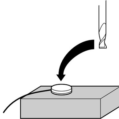
When the tool touches the sensor, the following message appears on the display and the amount of shift is set. After making the setting, the tool rises automatically.
