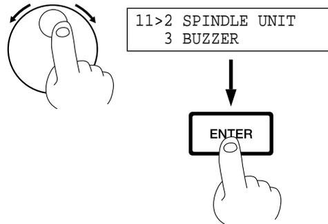
**4** Turn the dial to move the arrow to [HIGH TORQUE] or [HIGH SPEED], then press the [ENTER] key. The selected mode is enclosed in angle brackets.
