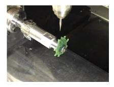
ProtoWizard's Ring Arbor has a unique triangular shape on the tip to locate the ring straight up every time. Positioning the ring is mistake-free with ProtoWizard. ProtoWizard's Core and Supports eliminate the guess work. Use ProtoWizard's Ring Arbor to cut those fine details 360 degrees around the ring.
