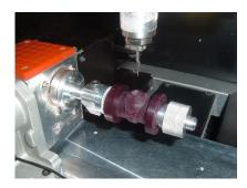
ProtWizard's Ring Tube Fixture locates on the center hole of the Ring Tube wax. Us any style or size of wax. Presize the hole and use ProtoWizard's Supports to eliminate the time consuming clean up.
