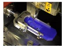
Extend the cutting area for longer pieces such as Ear Rings or Pendants using the ProtoWizard Extension Supports with the Flip Fixture. Made from precision aluminum, the Extension Supports have little "ears" out on the end to compress an stiffen the wax. This eliminates and bending or warping of the wax.
