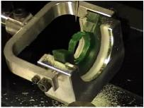
Flip the fixture up and machine +/- 60 degrees in bot directions
