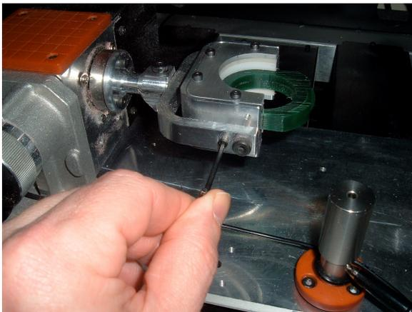
Using the hex wrench provided, loosen the small screw on the left of the pivot bolt. Back this out until the inside fixture can be pulled toward you and flipped vertical.
