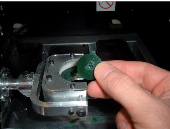
Once the program has completed and the spindle has stopped, remove the part from the wax by breaking it from the supports holding it in the blank wax
