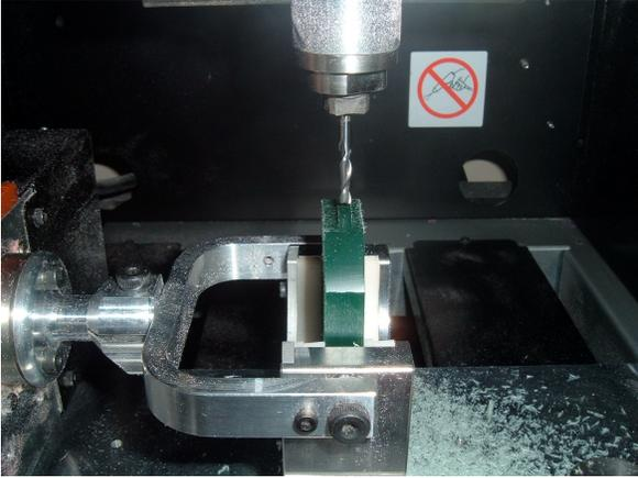
Jog the X axis over the center of the 1/8" channel. Center the 1/8" Tool directly over the 1/8" channel by jogging only the X axis.
