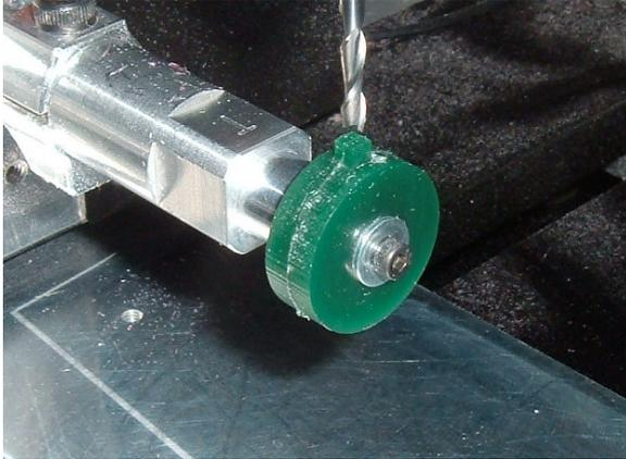
Jog the A axis to rotate the part to align the 1/8" square under the 1/8" tool.
