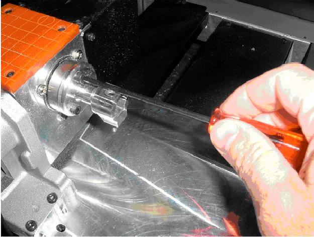
Using the three screws provided, carefully install the Rotary Adapter into the rotary table face. This should be a snug fit. Caution should be taken to not have this crooked. Gently rotating the adapter in the counter bore of the rotary table will help. Insert all three screw finger tight before tightening with the provided allen wrench.
