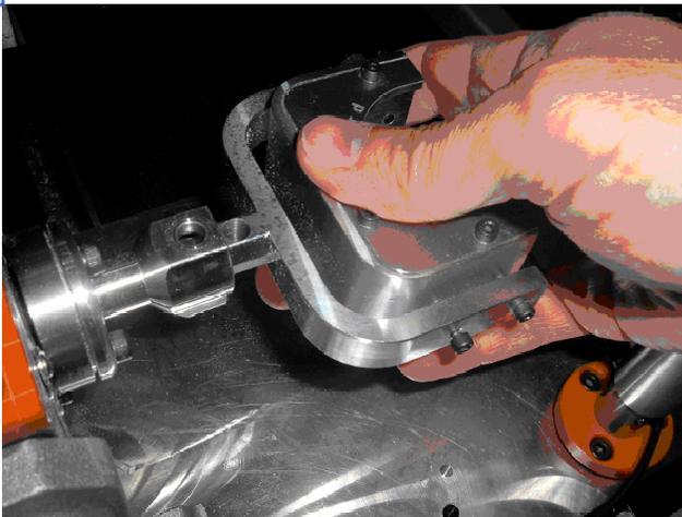
Carefully insert the 3-Sided Flip Fixture into the Rotary adapter making sure the holes align in the center of the 2 parts.
