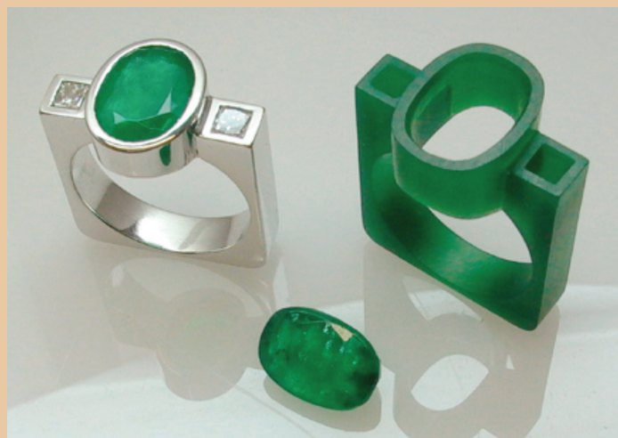
Finished ring produced from wax model made with MDX-540.
