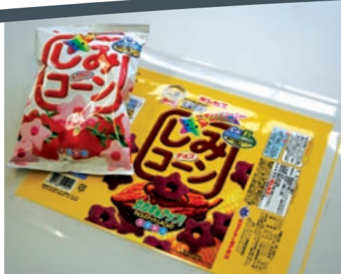
Packaging prototype produced on the Roland LEC-300 (right) along with final package (left).
