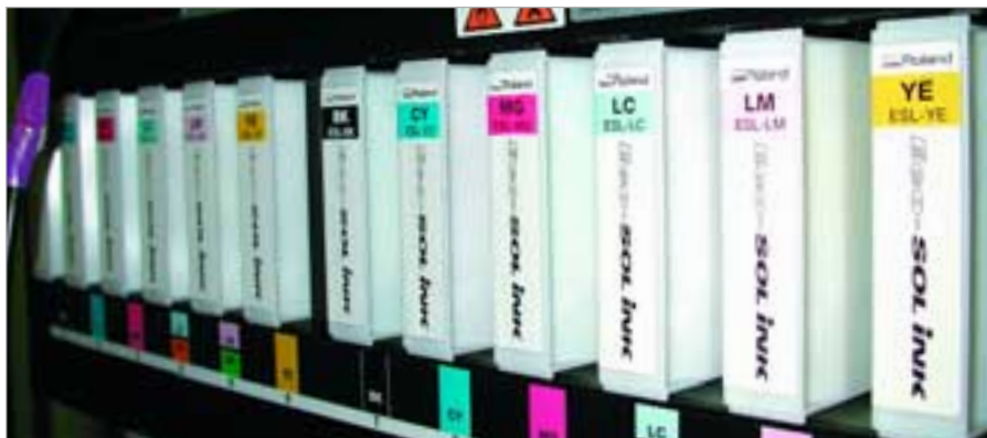
Figure 1: Roland's Eco-Solvent ink uses dual ink cartridges that boost the ink delivery system of the new SOLJET Pro II EX series. The Advanced Eco-SOL INK works in conjunction with an integrated media heating system to bond aggressively to economical media, including both coated and uncoated substrates.
