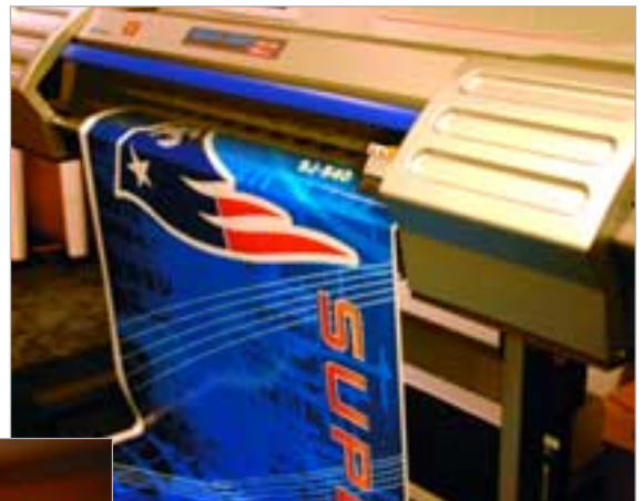
Figure 5: Printing on a variety of media was simple. The easy media loading procedure was the same for each media type, regardless of whether you were loading PSV, scrim banner vinyl or soft signage fabrics. For instance, when printing on Roland's FRSB Flame Retardant Scrim Banner, we adjusted the printhead height and produced P.O.P. graphics that doubled as translucent displays and banners.
