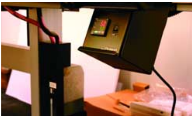
Figure 2: The heating unit on the SOLJET Pro II EX enhances the fixation of the Eco-SOL INK on the media and dries ink faster by preheating the media before printing. The controller allows users to adjust the heater temperature to match the media.
