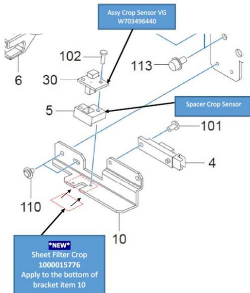
Bottom view of the cut carriage assembly.
