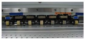
The pinch rollers may be easily removed through the channel identified by the arrows when not in use.
