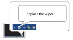
The wiper is a component used for cleaning the print heads. When the message shown in the figure appears on the Utility icon on the computer task tray, it is time to replace the wiper with a new one.
