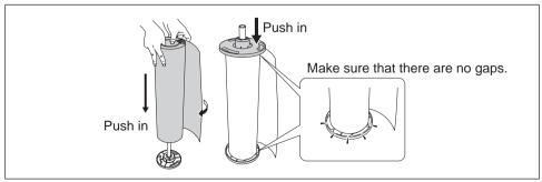
Place the roll media loaded onto the media bar on the printer.
