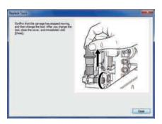
If the screen shown in the figure appears, open the front cover and replace the blade.
