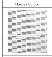
Dust and dirt stick to the print heads and prevent normal discharge of ink.
