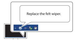
The felt wiper is a component used for cleaning the print heads. When the message shown in the figure appears on the Utility icon on the computer task tray, it is time to replace the wiper with a new one.
