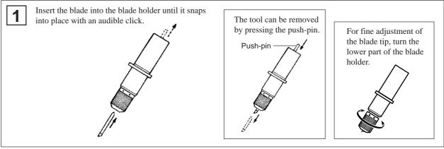
Insert the blade holder into the tool adapter. Then, depending on the thickness of the material to be cut, insert the spacer or spring included with the tool adapted, or attach the cap without inserting either the spacer or the spring. Cap Blade holder Cutting force Fluorescent and 1 kgf reflective sheets, etc. Spacer Cutting force Sheets for indoor/ 80 gf outdoor use, etc. Spring Cutting force Sheets for outdoor None Tool adapter 35 gf use, etc.
