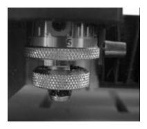
6. Lower the spindle down onto the surface of the material by pressing the **spindle** key on the control panel. Take care not to "over travel" the spindle downward as this will cause an error. As soon as the bottom of the nose cone touches the surface of the material, take care in lowering the spindle down further-- but only a small amount.
