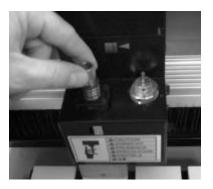
5. Ensure that the nosecone is turned "counter-clockwise" almost all the way down. The ratchet sound heard from the ball clicking into the indentations on the micrometer ring will disappear if you turn the ring to far.
