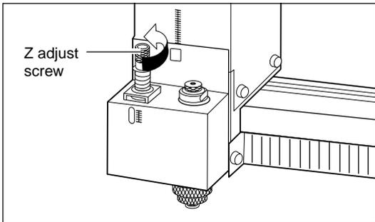
**4** Press the arrow keys and the [-Z] key to move the tip of the depth regulator nose to the surface of the workpiece.
