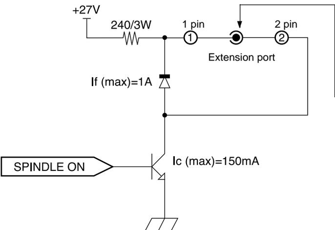
This circuit is activated when the spindle motor is in operation.
