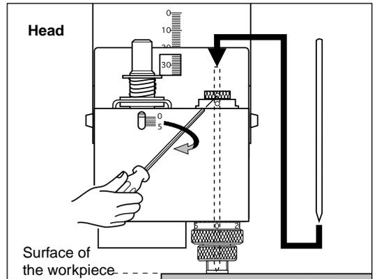
**7** Raise the spindle with the [+Z] key.
