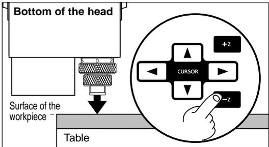
If the depth regulator nose does not reach the surface of the workpiece even when the [-Z] key is held down, rotate the micrometer dial in the direction shown by the arrow in the figure to extent the tip of the depth regulator nose to the workpiece surface.
