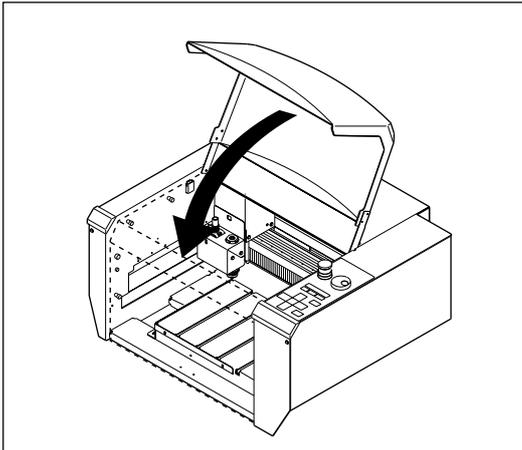
**4** Press the [SPINDLE ON/OFF] key to rotate the spindle.
