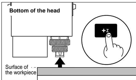
**8** Rotate the dial in the direction of the arrow shown in the figure to extend the cutter to the engraving depth (cutting-in amount). Move the cutter out just enough for the necessary engraving depth. The lines printed on the dial indicate 0.0254 mm (0.001 in.) for each mark. For instance, to set a cutting depth of 0.5 mm (0.0197 in.), rotate an 20 mark portion.
