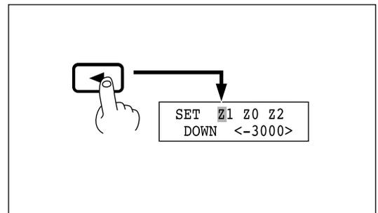
**5** Press the arrow keys and the CUTTER UP/DOWN keys to move the cutter to the height where Z1 (or Z2) point is to be set. When setting Z1, move the cutter to a position away from the loaded workpiece.
