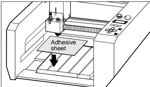
**2** Place the workpiece to be cut on the adhesive sheet and fasten it while pressing down.
