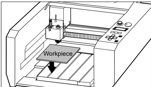
**2** Slide the square portion protruding from the bottom of the clamp plate into the groove on the table to secure the workpiece in place.
