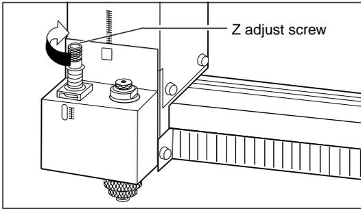
**2** Press the arrow keys and the [-Z] key to move the tip of the head to a position close to the surface of the workpiece.
