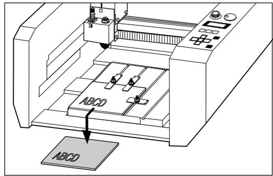
If the material has been secured in place using an adhesive sheet or double-sided tape, peel it off of the bed.
