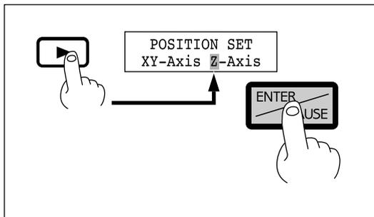
**4** Press the [◀] key to move the blinking cursor ("█") to "Z1." When setting the Z2 point, press the [▶] key to move the blinking cursor ("█") to "Z2."
