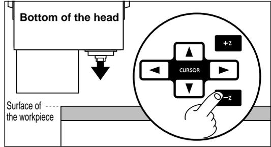
**3** Insert the cutter into the hole in the cutter holder and position the tip so that it gently touches the surface of the workpiece. Use the hexagonal screwdriver that comes with the machine to tighten the cutter mounting screw.
