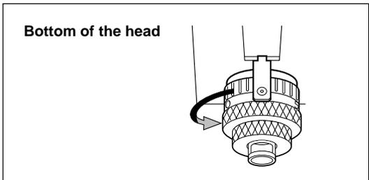
**5** Use the height setting made in step 4 to set Z0. Z0 is the reference point for raising and lowering the spindle. Refer to “Setting the Z0 Position.”
