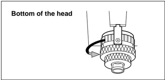
**3** Loosen the Z adjust screw.
