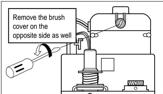
**4** Remove the old motor brush and replace with a new one.
