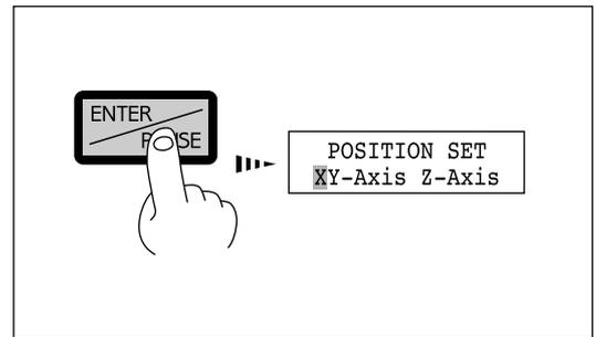
**3** Press the [▶] key to move the blinking cursor ("█") to "Z-Axis," then press the [ENTER] key.
