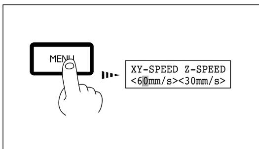
**2** Press the [◀] or [▶] key to move the blinking cursor ("█") to the value for the X-Y axes. To set the machining speed of the head, move the blinking cursor ("█") to the value for the Z axis.
