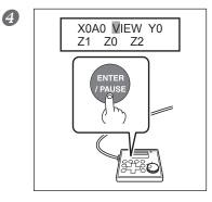
When engraving ends, move the spindle head to the VIEW position.
