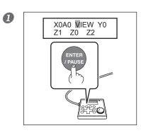
Close the front cover and move the spindle unit to the VIEW position. When movement ends, open the front cover.
