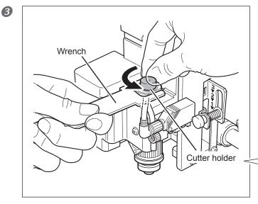
Open the front cover and install the cutter holder.
