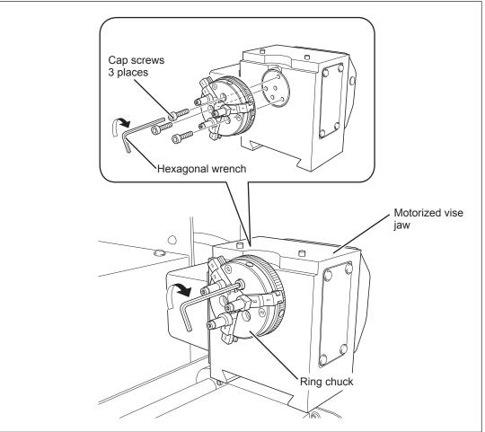
SAssemble the ring chuck to match the engraving method, then install the ring chuck. P. 93, "Using the Ring chuck"
