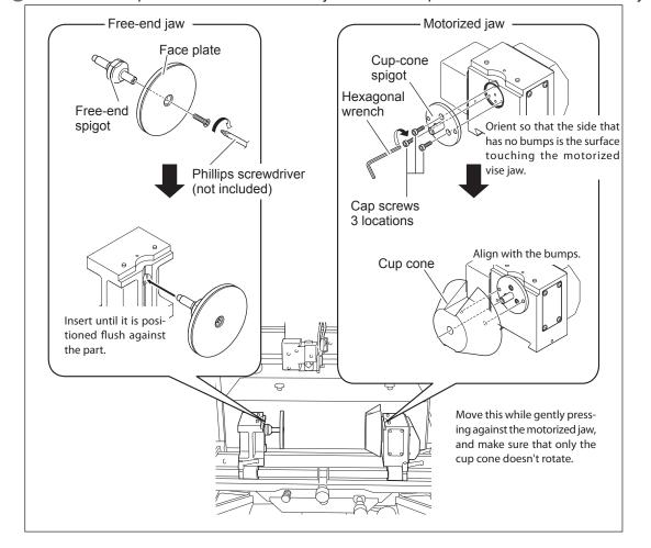
S Install the face plate on the free-end vise jaw and the cup cone on the motorized vise jaw.
