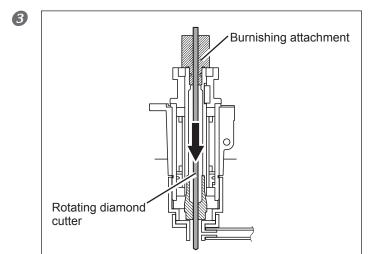
Insert the rotating diamond cutter into the burnishing attachment.
