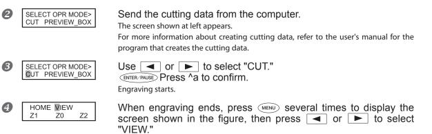
The spindle head moves to the VIEW position.
