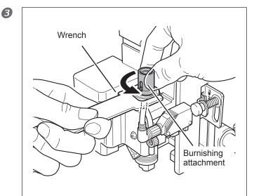
Open the front cover and install the burnishing attachment.
