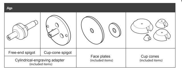
\*At factory shipment, the free-end spigot, the cup cone spigot, the face plate (100mm) and the cup cone (140mm) are attached to the main unit. S
