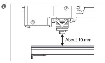
Use , , , , and , and to move the spindle head to the area above the workpiece, then press  $\sqrt{-z}$  to lower the spindle head. Stop at a position where the tip of the solid collet is approximately 10 millimeters from the surface of the workpiece.
