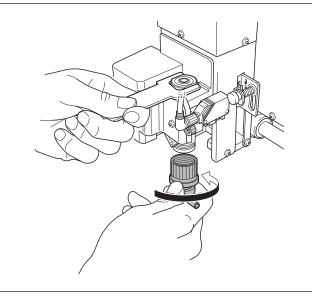
Tighten until no further movement is possible, then adjust so that the hose attachment port is on the right side as seen from the machine.
