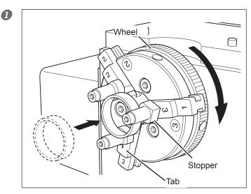
Place the ring inside the tabs of the ring chuck and butt it flush against the stoppers.
