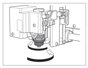
Tighten until no further movement is possible, then loosen two turns.
