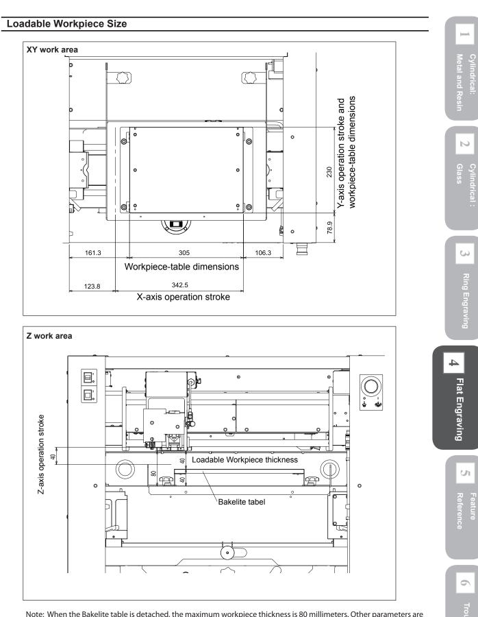
Note: When the Bakelite table is detached, the maximum workpiece thickness is 80 millimeters. Other parameters are unchanged.
