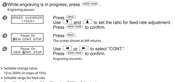
X- and Y-axis directions: 0.1 to 60 mm/sec (0.004 to 2.4 in./sec) Z-axis direction: 0.1 to 30 mm/sec (0.004 to 1.2 in./sec)
