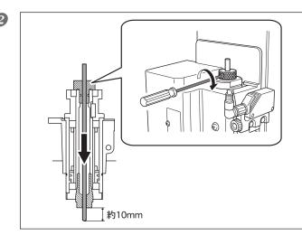
Tighten the mounting screw for the cutter holder, and secure the diamond scraper in place.
