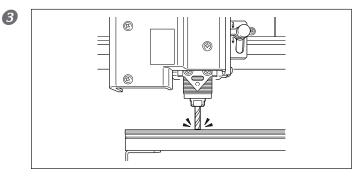
Press  $\sqrt{-z}$  to lower the end mill to a location where the workpiece is cut by a slight amount.
