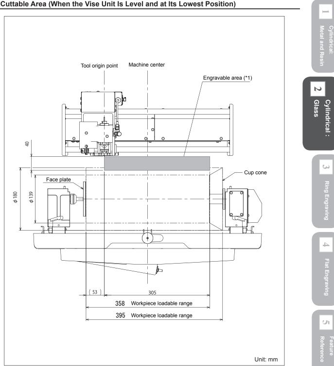
Cuttable Area (When the Vise Unit Is Level and at Its Lowest Position)
