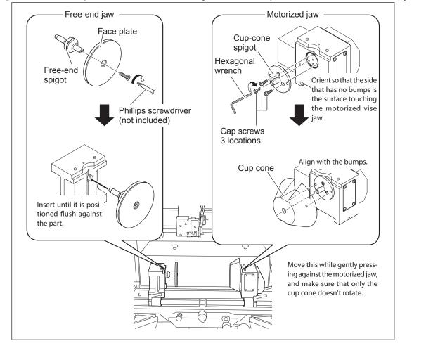
S Install the face plate on the free-end vise jaw and the cup cone on the motorized vise jaw.
