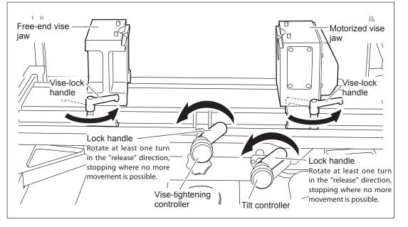
\* At factory shipment, the cup cone spigot and the cup cone (140mm) are attached to the motorized vice jaw, and the free-end spigot and the face plate (100mm) are attached to the free-end vice jaw. This illustration shows the state where each jig has been removed.
