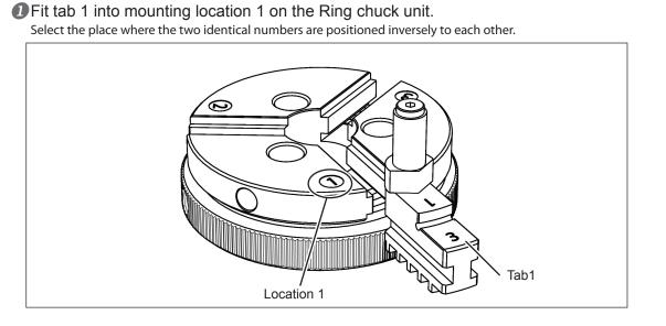
Rotate the wheel on the Ring chuck unit so that the teeth on the tab engage fit onto the rim of the wheel.
