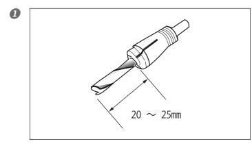
Insert the end mill into the end-mill collet.
