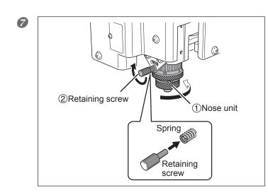
Make the setting for the cutting-in depth. (1) Tighten the nose unit to match the desired cutting-in depth. The amount of extension of the cutter is the cutting-in depth. 1 scale tick = 0.0254 mm 1 turn = 0.635 mm (4 to 8 scale ticks are approximately 0.1 to 0.2 mm) Secure the nose unit in place with the retaining screw.
