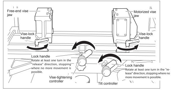
\* At factory shipment, the cup cone spigot and the cup cone (140mm) are attached to the motorized vice jaw, and the freeend spigot and the face plate (100mm) are attached to the free-end vice jaw. This illustration shows the state where each jig has been removed.
