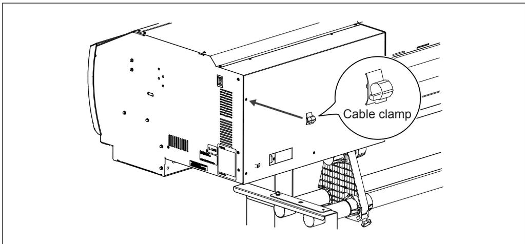
**2 Connect both the power cord and the Ethernet cable (commercially available).**
