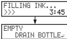
**When the screen on the left is displayed, discard the discharged fluid from the drain bottle.**
