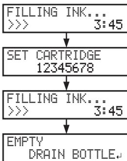
**When the screen on the left is displayed, insert ink cartridges into the slots whose numbers are flashing.**
