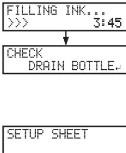
**When the screen on the left is displayed, make sure the drain bottle is not overflowing with discharged fluid, and then press
