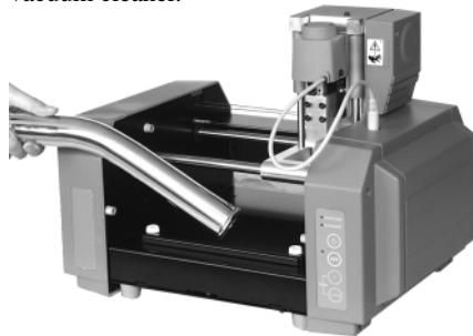
**4** Lift up MODELA and also remove any cuttings that may have fallen underneath.
