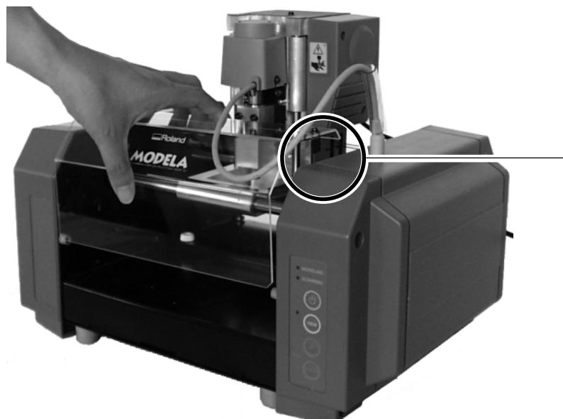
Fit the cover plate into place from above so that it goes into the portion shown in the figure.
