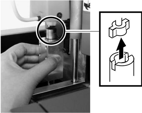
**6** lift up the spindle until it touches, and while holding the spindle in that position, use the included hexagonal (size : 3 mm) wrench to loosely tighten the screws you removed in step 1.
