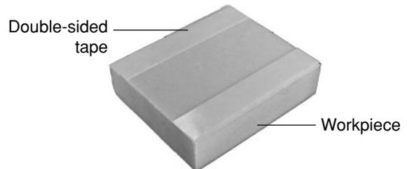
**3** Mount the workpiece with its corner aligned with the position of the work plate in the figure.
