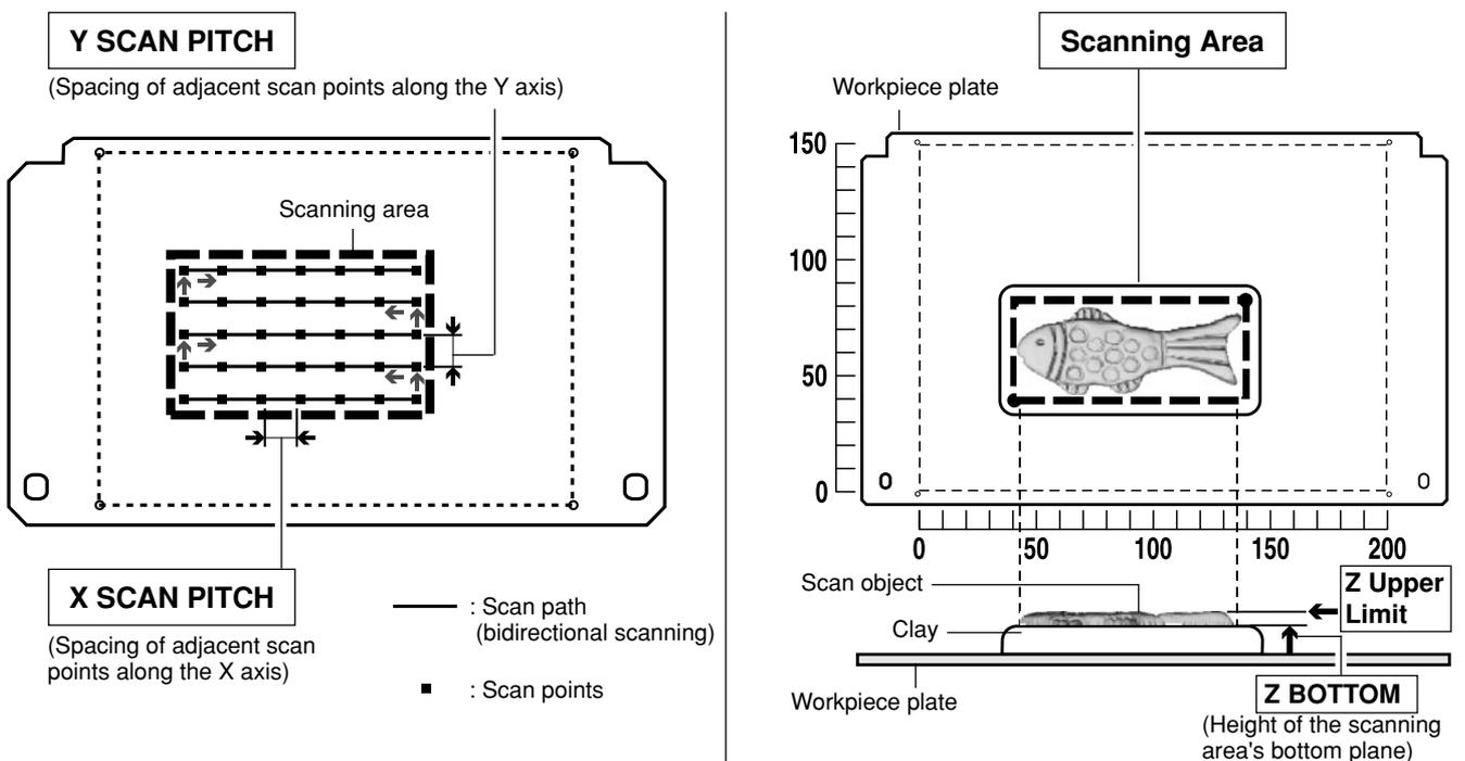
\* If you have made a clay base, the height of the clay is taken to be the Z-axis reference surface.
