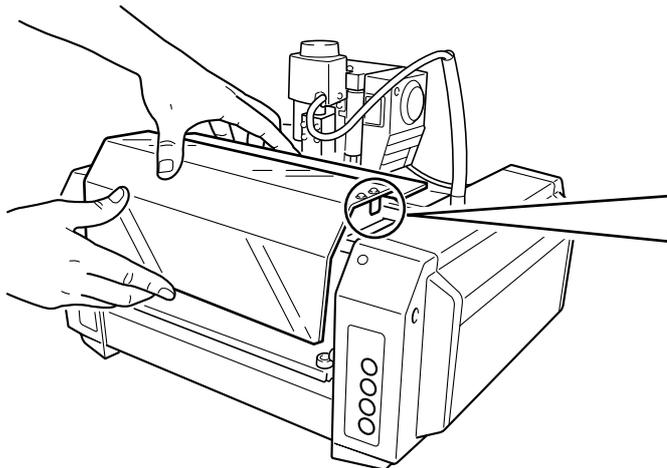
Fit the cover plate into place from above so that it goes into the portion shown in the figure.
