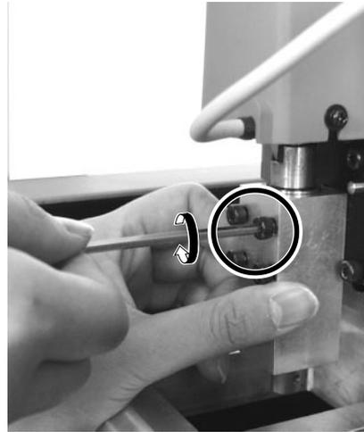
**7** After all four screws are in place, While supporting the spindle by hand, tighten securely.
