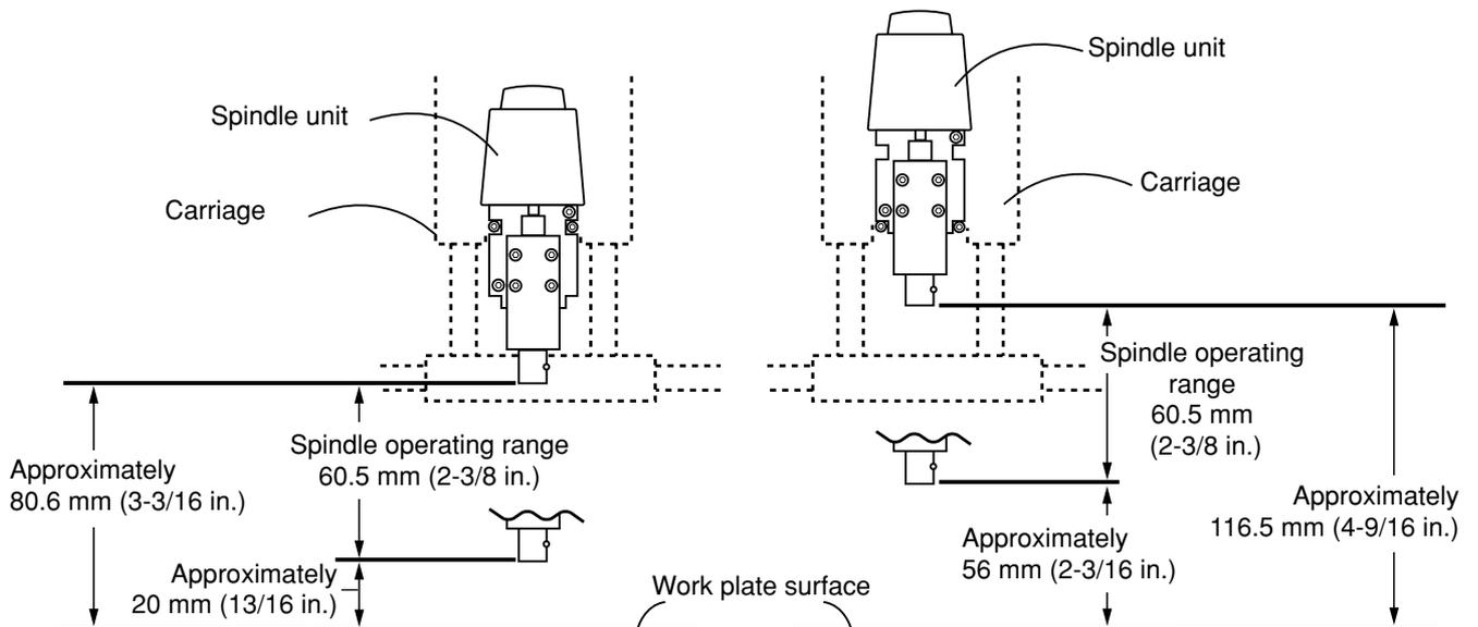
Load the material and install the tool. When using a base to load the material, mount the base as well.
