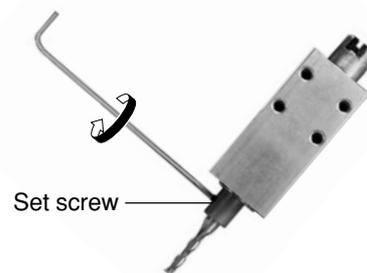
**5** Fit the spindle into place as shown in the figure.
