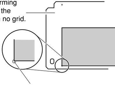
The center of the hole at the lower left of the work plate is the suggested X- and Y-direction machining reference point for Modela.
