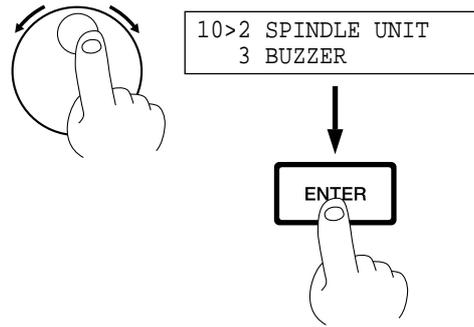
**4** Turn the dial to move the arrow to [HIGH TORQUE] or [HIGH SPEED], then press the [ENTER] key. The selected mode is enclosed in angle brackets.
