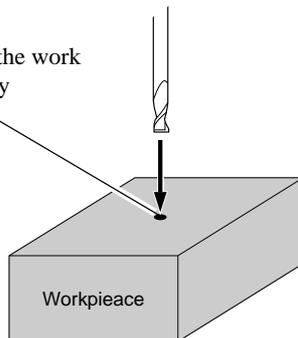
Press the [SPINDLE] key to make the spindle rotate. Place the tool in the marked position, then lower the tool until the ink is cut off. The ink mark on the work surface has a certain thickness, so only the ink is removed.
