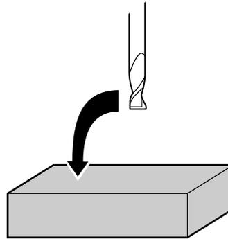
**3** Turn the dial to align the tip of the cutting tool with surface of the workpiece.
