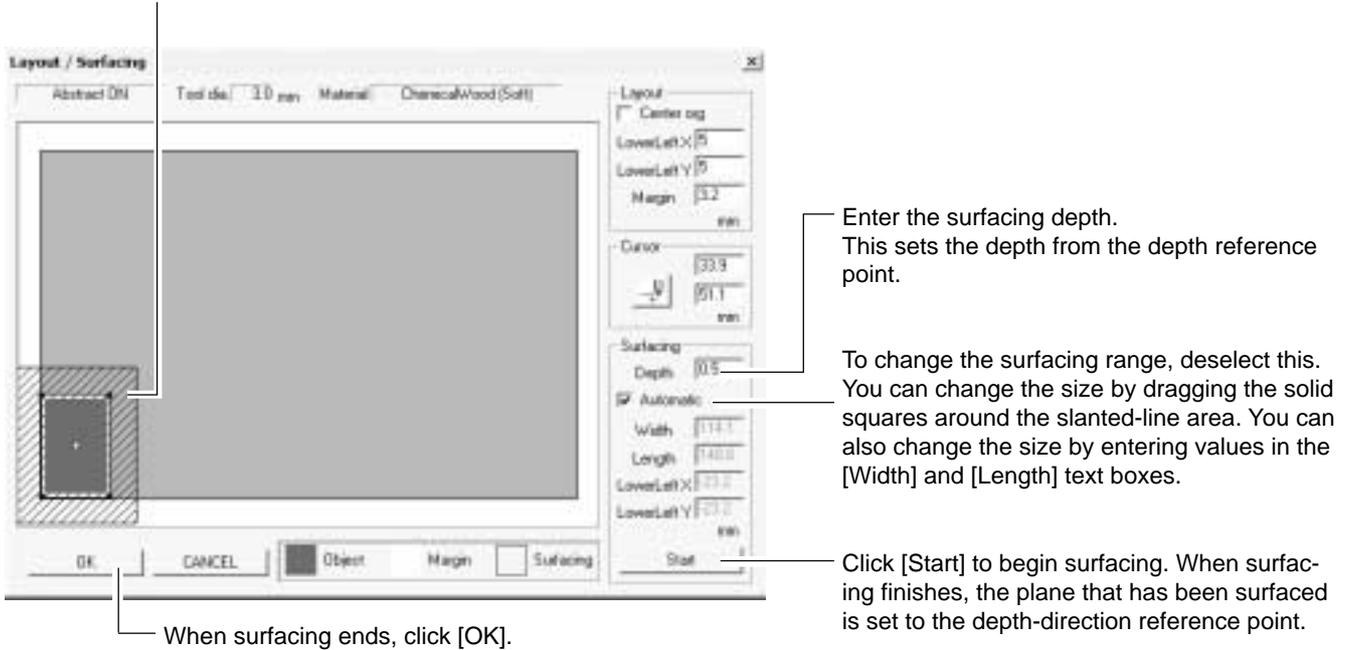
When surfacing finishes, MODELA Player and the coordinate view on the MDX-650/500 automatically sets Z0 on the surface of the workpiece after surfacing.
