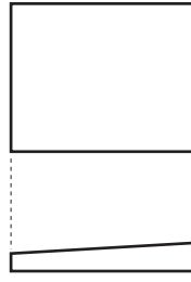
Surface to mark is not straight.
