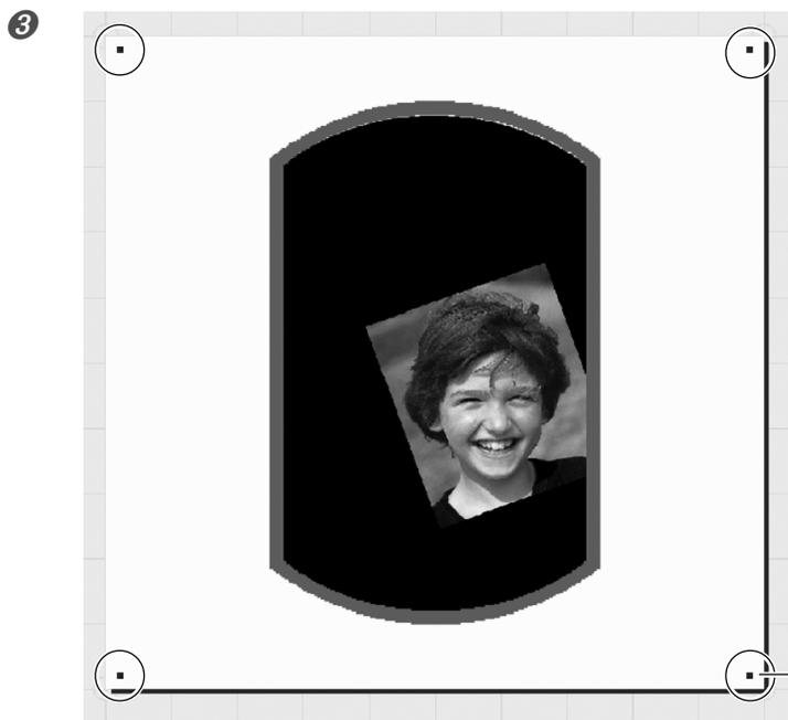
Drag the Handles (■) around the frame to adjust its size and location.
