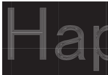
Island Fill You can specify the interval between adjacent filling lines.
