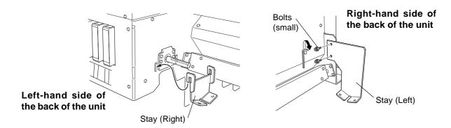
**2** Place the media guide on the stays and secure it in place using the included small bolts.
