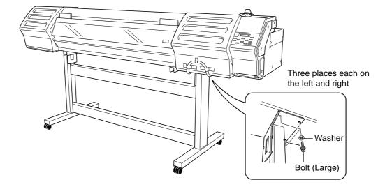
$\mathbf{3}$  Use the included large bolts to secure the machine to the stand.
