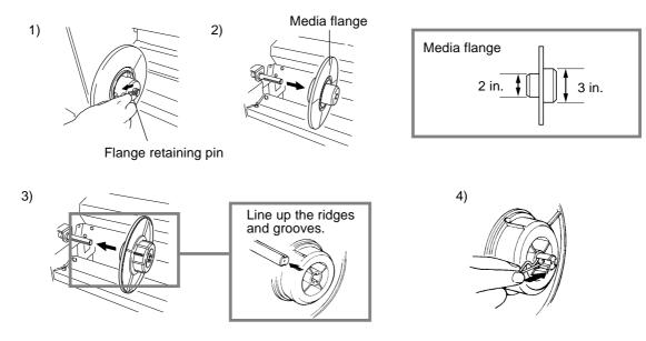
**3** Fit the hole on the left side of the roll media all the way onto the left-hand media flange.
