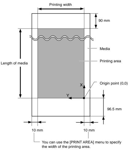
The media-cutoff location that is used when a media-cutoff command is sent from the computer is determined as follows.
