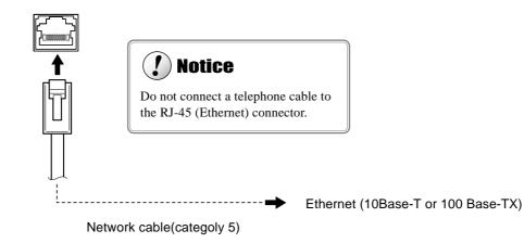
Various settings are required when using this machine in a network environment. For more information, see the "Roland PrintServer Network Settings Guide".
