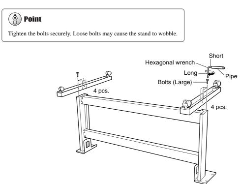
2 Set the stand upright so that the casters are at the bottom, and place the machine on the stand. The front and rear of the stand are as shown in the figure.
