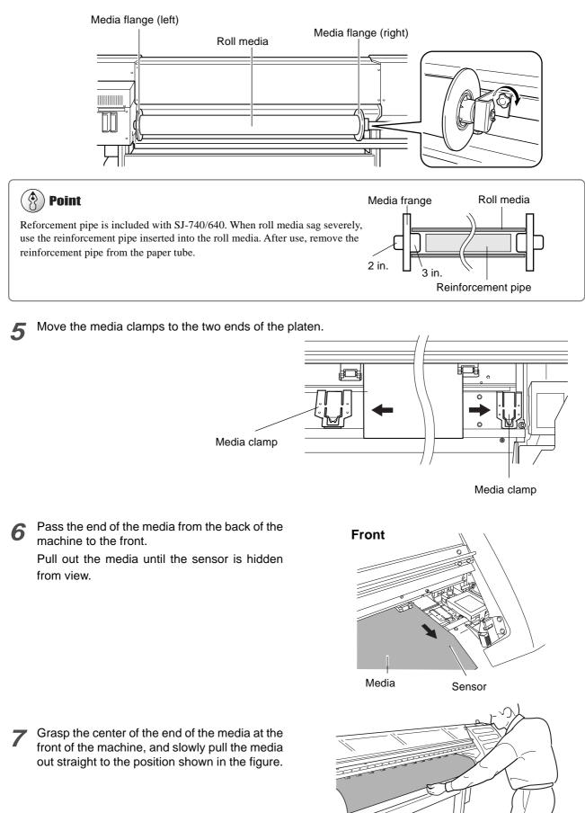
8 Slowly turn the media flanges at the back of the machine to pull back the media to the position shown in the figure.
