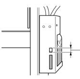
When the discharged ink is within this range, dispose of it. If discharged ink is allowed to exceed this range, it may
