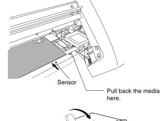
**9** With the media pulled out from the roll stretched taut with no slack, move the sheet loading lever toward LOAD.
