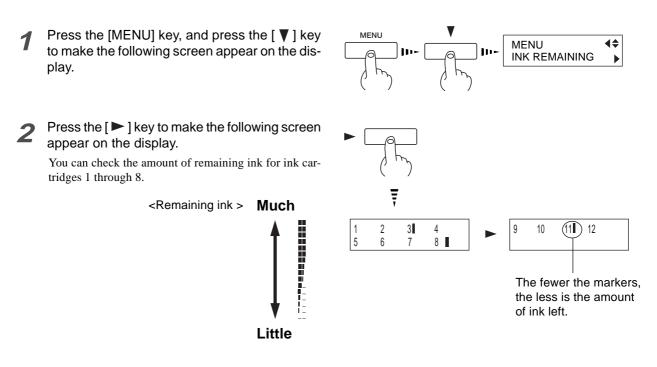
3 Continuing by pressing the [▼] key lets you check the amount of remaining ink for ink cartridges 9 through 12.
