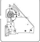
3 (high) : When media that is thick or prone to warping is loaded
