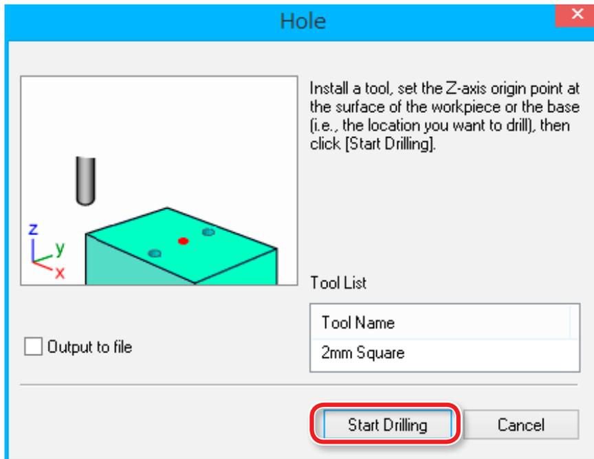
A dialog appears that shows what is being output and the progress of drilling.
