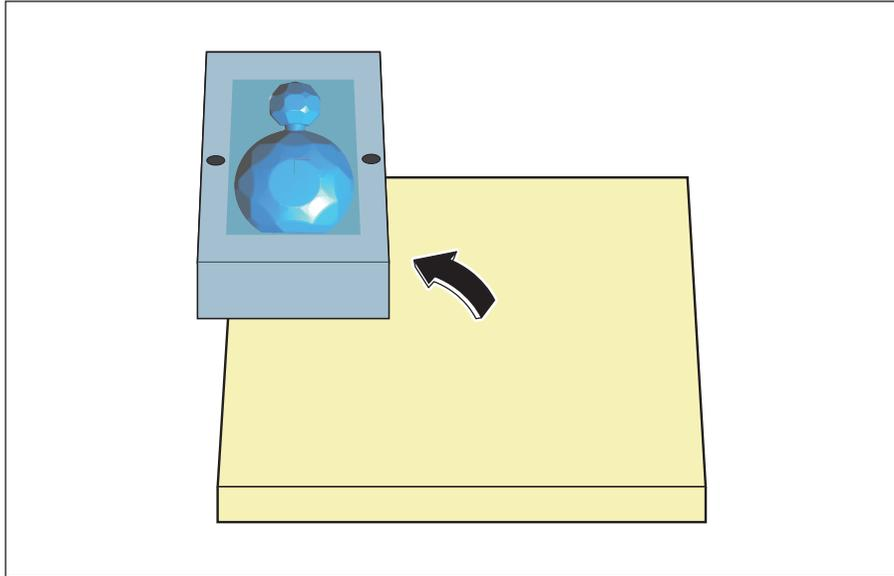
7. Make a mark on the material to ensure that you do not confuse the side to be reversed.
