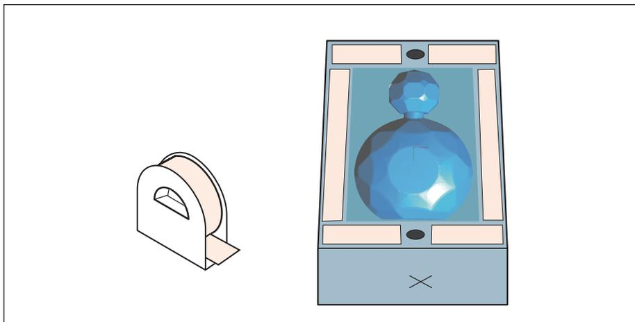
**5.** Rotate the material 180° toward you around the X axis and align the pins with the holes in the material.
