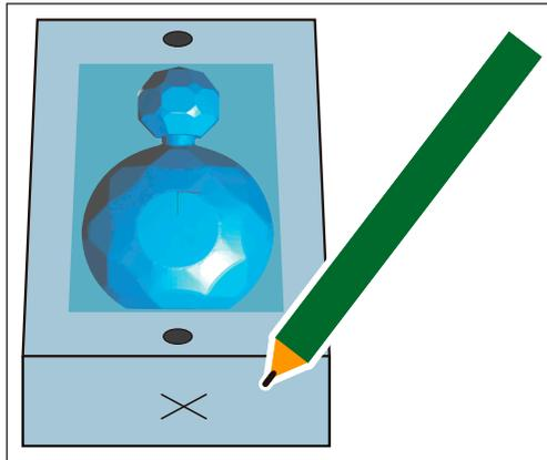
**4.** Adjust the Z origin so that it fits the scrap board while leaving the other origins intact.
