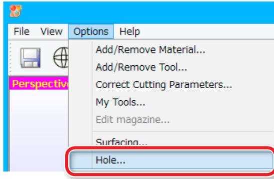
5. Configure the positioning pin diameter, the number of holes, and other settings as appropriate.
