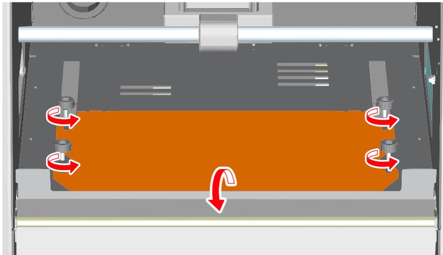
5. Affix the scrap board to the removed table, and slot the table under the screws.
