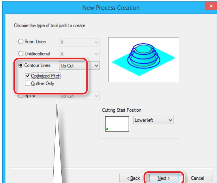
This Function enabled only in the finishing process.
