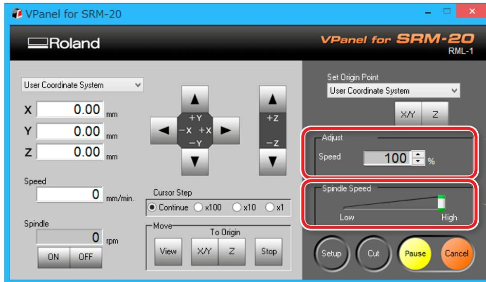
**Adjusting Cutting Speed (Override)**
