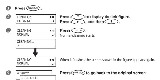
**Perform a printing test again to make sure the dot drop-out has been corrected.**If the problem persists, try performing cleaning a second time. If the printer has been used for a long period, the problem may persist even after two or three-cycle cleaning. Then try cleaning using a different method.
