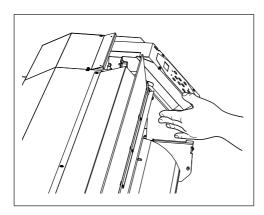
Touch the location shown in the figure to discharge any static electricity.
