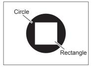
The test pattern is cut. Circle and rectangle are cut. Peal off the two shapes.
