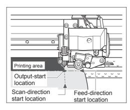
Use to to move the center of the blade with the output-start location.
