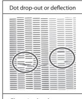
Flaws in the dot pattern are caused by dust on the print head.
