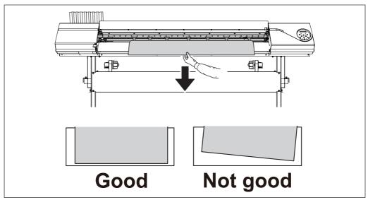
Dower the loading lever to secure the media in place.
