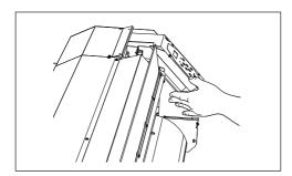
Touch the location shown in the figure to discharge any static electricity.
