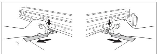
When you're performing cutting only using the roll media, never allow the media to hang down from the rear of the machine. (or set the [PREFEED] menu to "ENABLE.")
