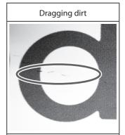
When dirt or dust accumulates on the print head it can interfere with image quality.
