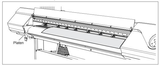
6 Check both edges of the media are placed on the grit rollers.
