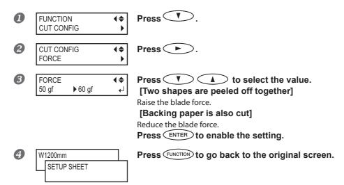
At the [CUT CONFIG] menu, you can also make settings for other cutting conditions in addition to the blade force. Refer to the following pages.
