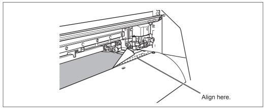
4 Lower the loading lever to secure the media in place.
