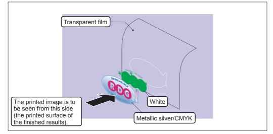
\* The white data and the metallic silver/CMYK color data are actually printed simultaneously, but they are shown here as separate layers in order to indicate the printing sequence.
