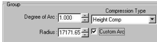
Custom Arc allows for specification of both the Radius and the Degree of Arc without regard for the actual length of the text being fit into the available space. This is accomplished by applying a Compression/Expansion routine to the text string to force it to fit onto the specified arc. There are three options available for fitting the text into the specified space: Height Compression; Width Compression, and Kerning Compression.
