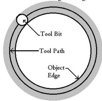
The tool path will fall to the outside of the artwork with an offset equal to one half the width of the tool bit. This type of offset is typically used to cut objects out of a piece of material.
