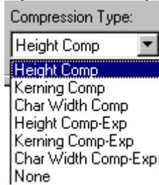
When using a compression type, specify a line width for the Compression function to operate. This length is specified under the Width option by entering a value in the Unit edit box.
