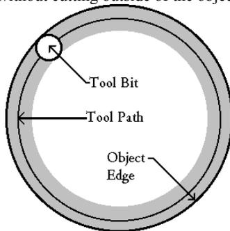
Tool Path will fall inside of the artwork with an offset equal to one half the width of the tool bit. This offset is typically used when filling or cutting out an object.
