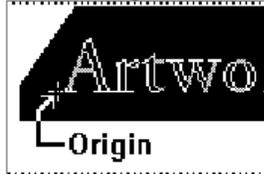
While this task can be accomplished by setting an X- and Y-move from within the Cut dialog box, jogging the plotter head offers a more precise setting. This is because the head of the router can physically be moved to the desired position before committing to the rout. Also, use the Jog option to change the angle of the baseline for a given rout.
