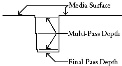
A Secondary Clean-up Pass will help you avoid this result. Selecting a Secondary Clean-up Pass will cause the router to trace once more around the edge of the cut object with the bit at full depth, leaving
