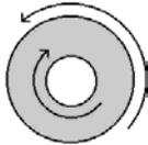
The proper use of this setting will ensure that outside edges are cut with both the tool bit and the tool path facing the cut. This will produce a clean, smooth-edged cut.
