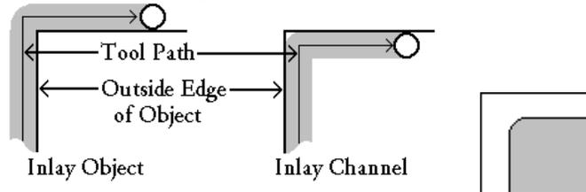
Resolve this problem by selecting Inlay. This will cause the router to cut all corners in an identically rounded fashion, so that all of the inlay pieces will fit into their routed channels.
