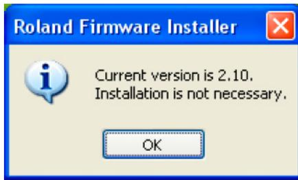
If the installer detects that the printer already has the version of firmware installed, it will display the above prompt. No upgrade is necessary.
