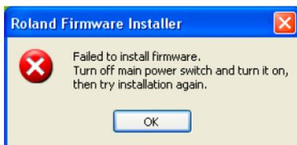
The "Failed to Send" and "Failed to Install" dialogs occur typically if there is a problem with the firmware itself, or the power is turned off during updating. Cycle the power of the printer and attempt updating again.
