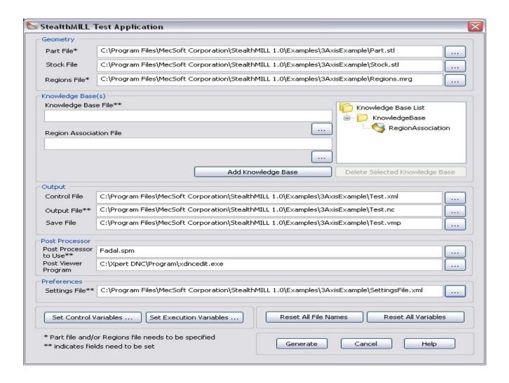
StealthMILL can also be run from the command prompt by giving a control file as input. A control file contains information about locations of various geometry files, knowledge base files to define Machining Operations, other control variables and execution variables. It is in XML format and is used to drive the StealthMILL application.
