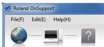
When the globe image linked to a computer is displayed, your computer is connected to the OnSupport server.
