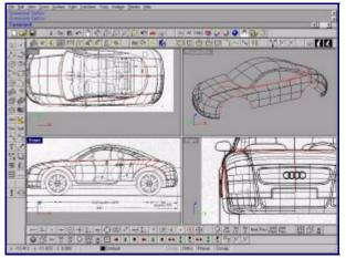
Create the top edge of the wheel arches, create the curve of the belt line at the bottom of the side glass. to create these curves flat using the existing geometry as reference as well as the images you can use the 'project to cplane' option in the Osnap box Project the three curves onto the side surfaces of the body (command: Project) and Split surfaces with projected curves.
