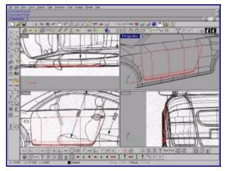
Use ExtendSrf to extend the lower part of the side surface to be able to create the door. In the front view draw the curve of the lower part of the door, project this curve on the enlarged surface, split the door with this curve of projection. Delete the extra parts of the body side. Now create a lofted surface (command: Loft) between the two lower door curves to create the chamfer.
