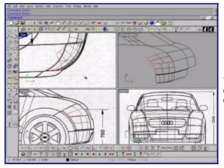
We'll begin the constructing the body side at the rear. Using the images in the top view and in the front view, draw curves delimiting the rear light and the lower part under the light. Create the surfaces with Sweep2.
