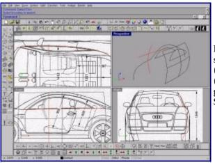
In the right view draw an arc corresponding to the radius of the side window, and in the top view draw the curve of the waist line (belt line). With these two curves create a one rail sweep surface (command:Sweep1). Project the curves of the drip line onto the glass surface and use these projected curves to split (command: Split) the surface.
