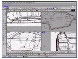
To finish off the side surfaces, we'll create the door and its small chamfer in the lower portion of the rocker panel. Draw the curve for the shut lines of the door in the front view, and project this curve onto the different surfaces of the body sides. Make a copy of body side surfaces. Split the copy of the body side, the rocker panel and the upper body side with the projected curve. Delete the internal part of the door.
