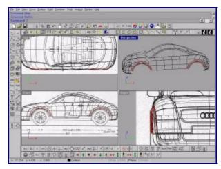
In the side view draw the front and rear wheel openings . Edit the curves, referring to background images, and then draw the wheel opening section curves. Use the Sweep2 command to create surfaces.
