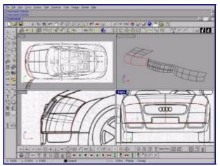
In the front view create curves for the roof, the windshield, the hood, the rear window,
