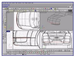
For the lower part of the front end build a "sweep one rail" between the lower edge of the front end surface created earlier and the profile curve that you created in the front view at the beginning of this tutorial.
