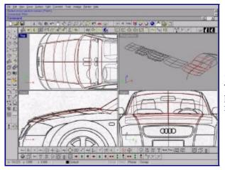
For the windshield another one rail sweep will do the job (command: Sweep1) with the curve that you drew in the front view and the edge of the surface of the roof that you made in the previous step. Edit its control points to widen it. Use the same method to form the hood.
