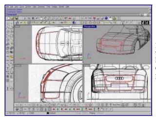
Finally, we'll to add a few details to the front end. In the right view, draw the characteristic curves of the main parts, headlights, the front grill, air intake etc. Project all these curves on the different surfaces of the front end. Split surfaces with the projected curves.
