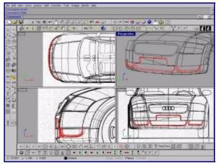
For the air intake and the license plate create ruled surfaces with the Extrude command, "T" option for Tapered, enter a value of angle, a distance and Enter. Create the surface of the license plate with a patch surface (command:Patch)
