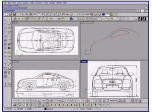
In the front view create curves for the roof, the windshield, the hood, the rear window, and the front and rear bumpers.
