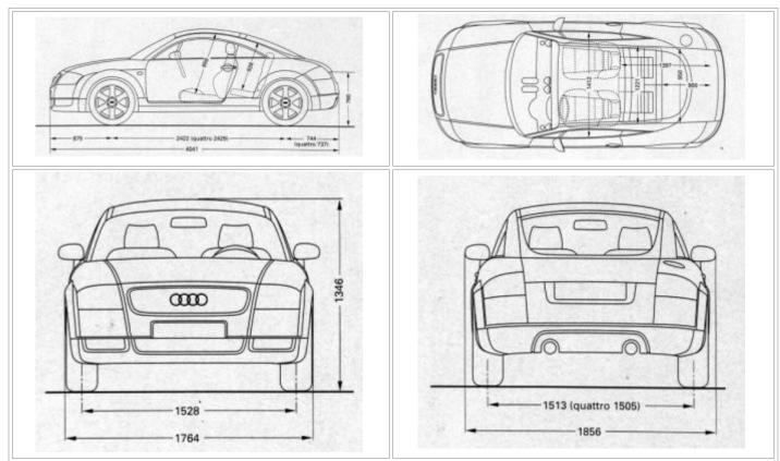
Once the images are in place, we will draw the characteristic curves of the car. Try to make the curves as "clean" as possible, meaning that the number of control points is reduced a minimum that will accurately define the curves. This will help to avoid inflections or waves. The quality of your initial curves will largely determine the quality of your final surfaces. Without beautiful curves you may have problems later with lights and reflections on your car's surfaces during rendering.
