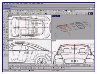
Use the curves of the front view of the roof and of the rear window to create extruded surfaces (command: Extrude; Option 'B' - for both sides). The extrude command having given us a surface of degree 1 with 2 control points, we must reparameterize the surface to degree 3 with 4 control points(command: ChangeDegreeSrf). We can now edit the surface by its control points to curve the roof and the rear window, using the background images in the three views as references
