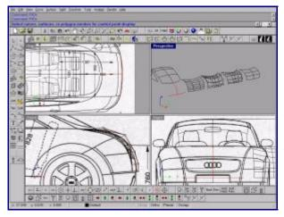
For the rear part create a curve in the top view representing the end of the boot, then create a "sweep one rail" surface (command: Sweep1) between the edge of the rear window and this curve. If the resulting surface has a lot of control points, use RebuildSrf to reduce the number of points. Edit the surface points to obtain the correct form
