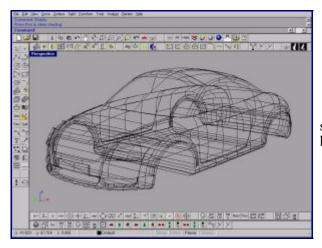
Make sure the surfaces are symmetrical and finally create a surface lofted surface going joining the wheel opening on the the left to "close" the volume for the rendering.
