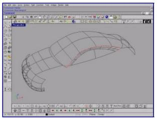
Lets move on to the side surfaces. For the A-pillar and the drip channel, we'll create two cross section curves: one between the lower edges of the side glass and the lower edges of the windshield and then one between the lower wdges of the side glass and that of the rear window using the curve blending tool.(command: Blend) Make a "sweep two rails" by using these curves as "cross sections", and the upper edge of the side glass and the edge of the roof/windshiels surface as rails.
