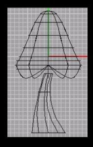
Now you want to fillet the edge of the bottom of the stem. Type "cap" and select the stem. This will cap the open ends and make it an edge that can be filleted. Type Flte and select the edge that you want to fillet. Give it a radius of 1 to make it nice and smooth.
