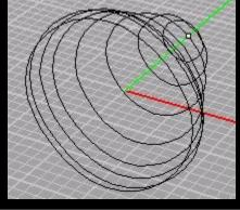
Now type prepcurves and make sure all the arrows are lined up. Use 5 control pts. Then loft the curves. type loft; hit N, hit P, goto the snap toolbar and select point snap. Move your mouse over the point that you created, click, then click all of the curves down to the very base. From there, hit P again. This time you will want to create a point up inside of the cap to make the bottom concave.
