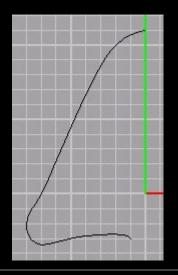
Once we lay out this curve, we want to make copies of it around it's central axis. To do this, go to a perpindicular viewpoint, and click rotate, hit C to make copies, and place a copy every 90 degrees. You will need gridsnap to do this correctly. If you don't know how to rotate, read the Rhino Users Guide available at www.rhino3d.com
