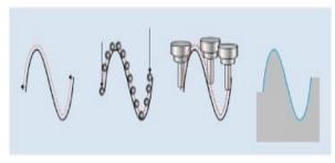
SRP Player Pro uses advanced polygonal smoothing technology to achieve especially smooth surfaces using STL files. It also takes IGES files and generates tools paths directly, without converting them into polygonal data.
