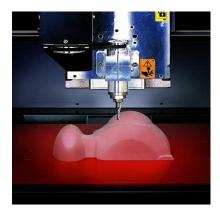
SRP (Subtractive Rapid Prototyping) – starting with a solid object and removing unwanted material – has several advantages over traditional 3D printing. Desktop milling machines cost significantly less than 3D printers, while producing prototypes out of a wider variety of non-proprietary materials with greater precision and better surface finish. The technology is also better suited for a wide range of custom rapid manufacturing applications.
