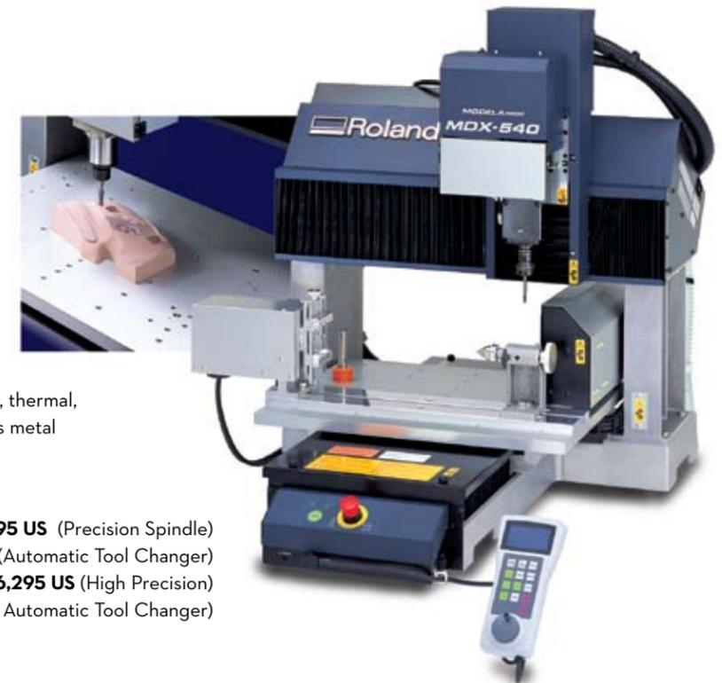
Roland 3D scanning and milling machines allow engineers and designers to quickly and inexpensively create 3D prototypes as well as wax models for jewelry design.
